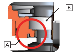
A Labyrinth structure B Dust-proof ball bearing
